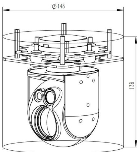
FIG. 1-1-1 Three-light integrated pan-tilt structure
